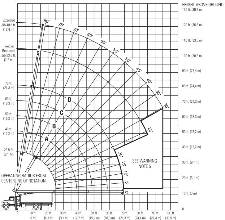
Lifting Capacities 3-section Boom 26.5 ft. - 70 ft. Jib 23.6 ft. - 40.6 ft.
